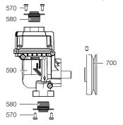
590 Pump 580 Flame arrestor protection 570 Fixing screws
