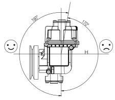
Figure 5: Installation position of the unit
