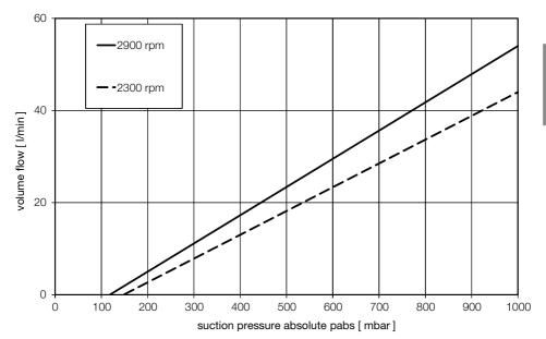
Figure 3: MEX 0831 volumetric flow rate characteristic curve
