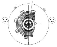
Figure 4: Installation position of the unit
