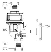
Figure 1: Spare parts for gas recovery pump MEX 0831
