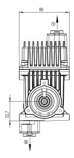
Figure 2: Dimensions of gas recovery pump MEX 0831
